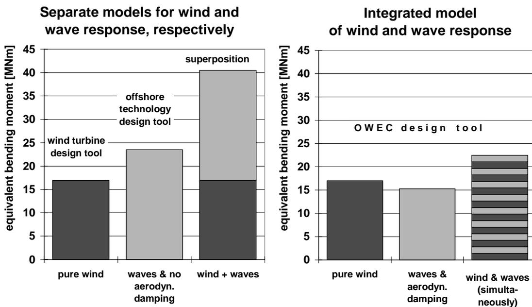
**Figure 7:** Reduction of calculated fatigue loading due to integrated modelling of wind and wave response (right) with respect to superposition of separate models for wind and wave response, respectively (left)
