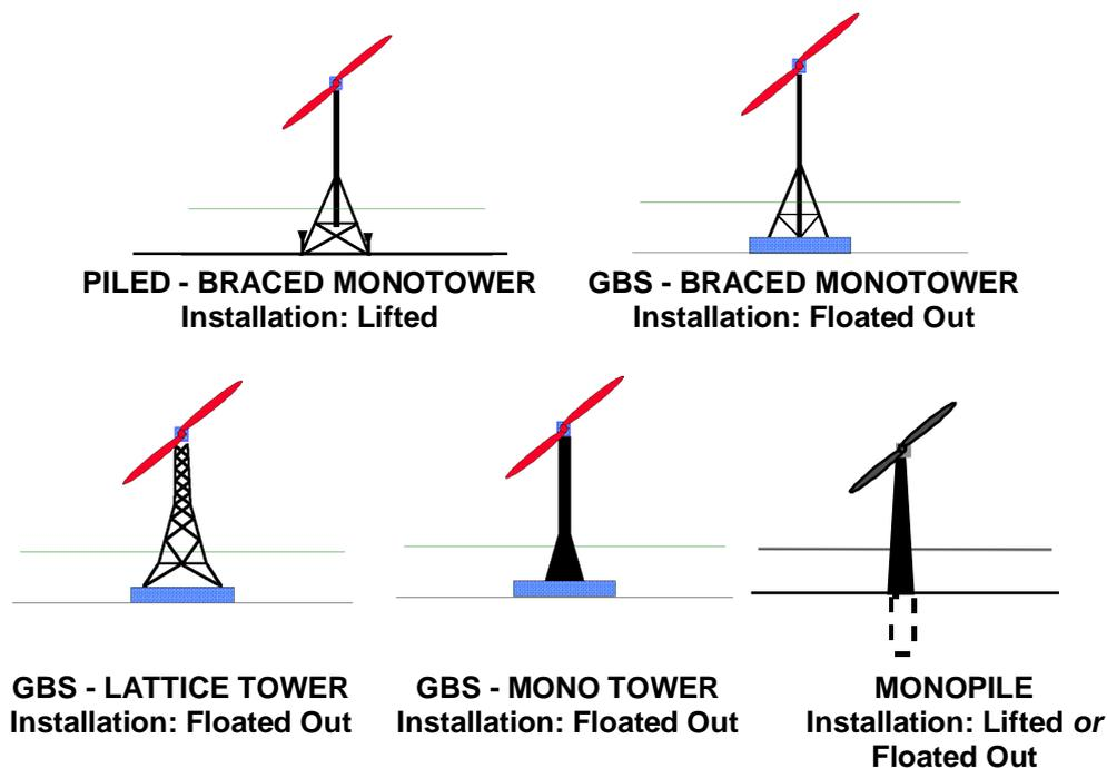
**Figure 13:** Examples support structure concepts
