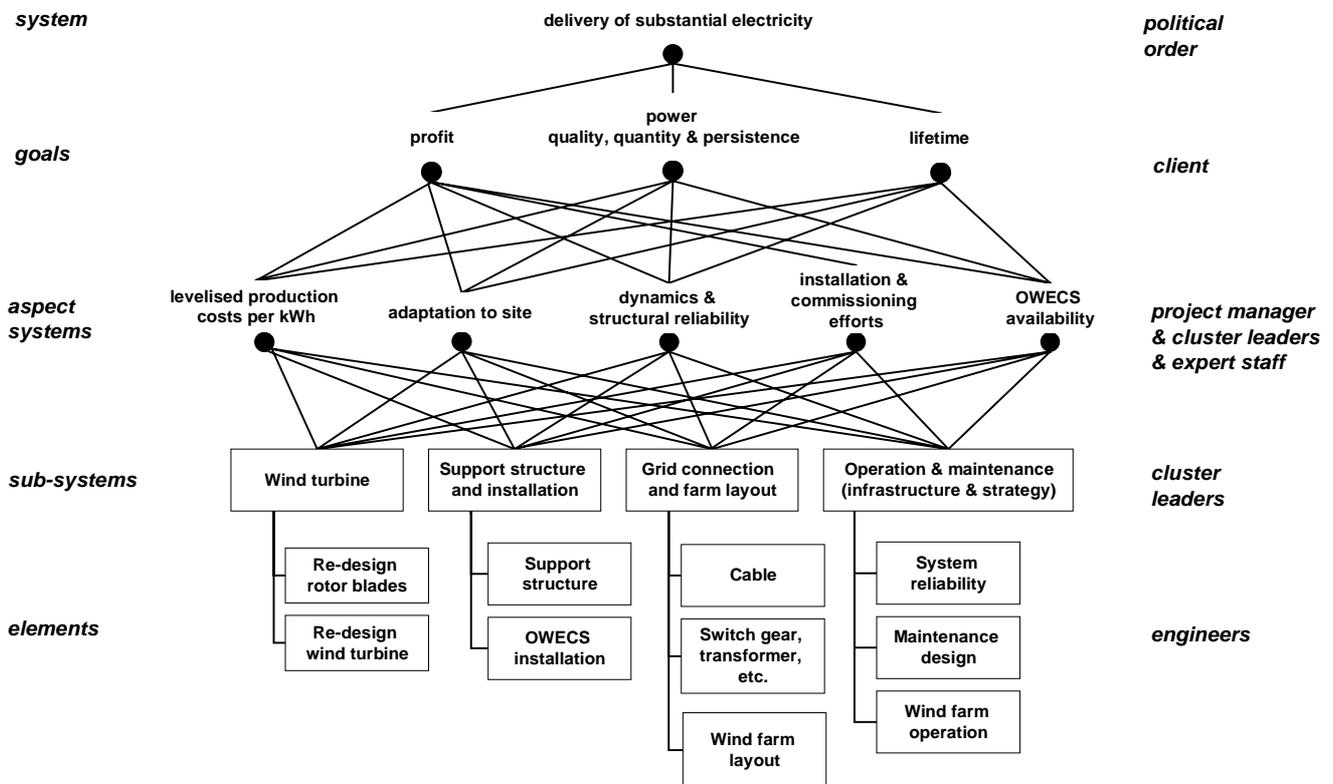
**Figure 3:** Multi-level control system within the integrated OWECS design approach
