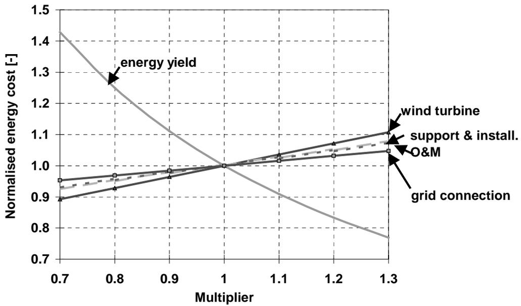
**Figure 17:** Sensitivity of normalised energy cost on (isolated) variation of sub-system cost, O&M costs and energy yield, respectively
