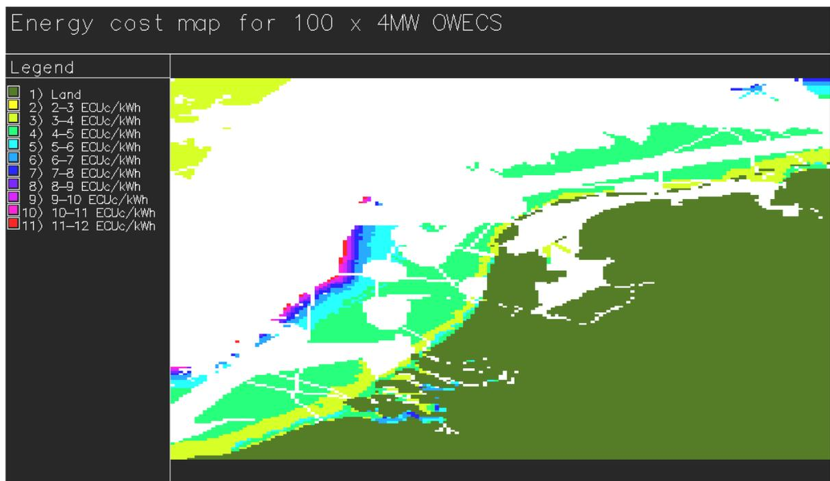
**Figure 12:** Energy cost map for OWECS employing 100 \* 1.5 MW units (above) respectively 100 \* 4 MW units (below) in Belgian and Dutch waters (Energy cost without onshore grid connection, for 20 years loan and 5% real interest rate.)
