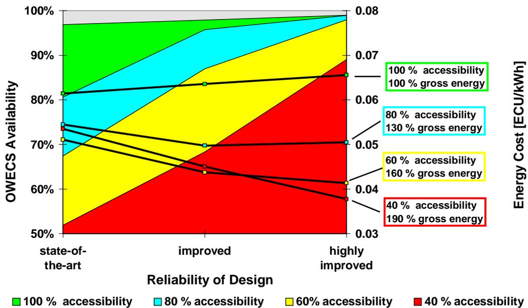
**Figure 5:** Qualitative relation between site conditions (accessibility and gross energy yield) on one hand and availability respectively energy costs for different level of reliability of OWECs design on the other hand
