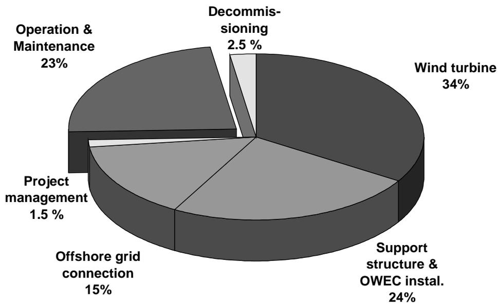
**Figure 16:** Contributions to energy costs of Opti-OWECS design solution
